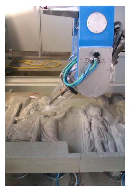
The bas-relief was machined in 90 deg. and in 45 deg. to reach the negative angles
