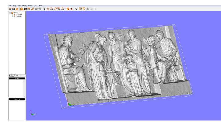
Model was scanned in at -z, -x and +x direction using Scantech 400mm scanner.
