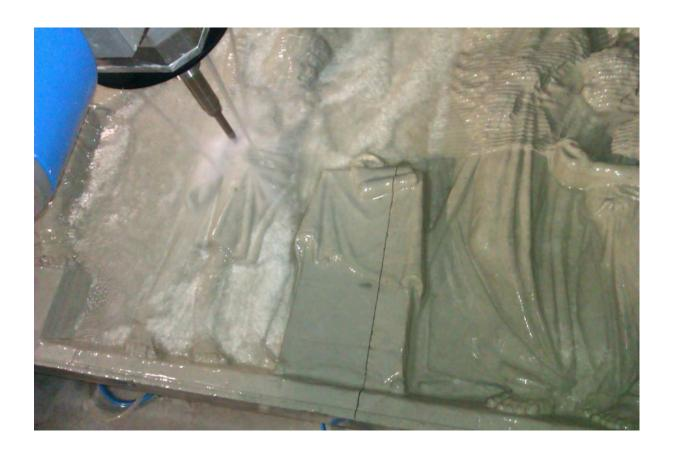
The final touches were done with conical tip mill Radius 3mm, step in Y in 0.8mm.
